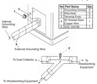
Make sure all machines are grounded with a 3 prong plug and that all duct & hose used to connect the collector to each machine are internally grounded.
