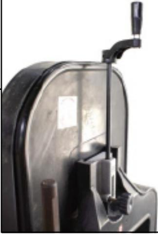
No one likes being under stress yet that is how we leave our band saw if we don't back off the blade tension.
