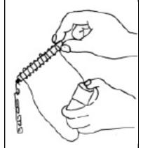
Using the small coil made in (3), insert the steel pin into the hollow plastic tube. Bring the compass near the tube and connect the wires to the battery case. Watch the compass movement. Reverse the battery connections and watch the compass' reaction.
