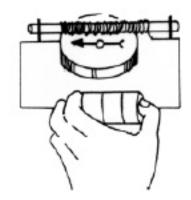
Make a small hollow coil be wrapping enameled wire around the small plastic tube. Remove the enamel from the ends of the wire for connection to the battery case. Place the compass under the coil as shown and connect the wires to the battery case. Watch the compass movement. Reverse the battery connections and watch the compass' reaction.
