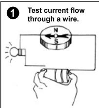
Position wire of light assembly over the compass. Connect the 2 wire ends to each terminal of the battery case. As the light illuminates, watch the effect of current flow through the wire on the compass direction. Reverse the connections to the battery and watch the compass direction again. Notice the compass direction as compared to the pole that the wire is connected to on the battery.
