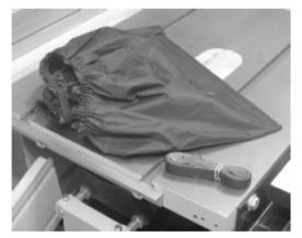
Clean all dust away from both sides of the saw body close to the opening in the back of the saw. Clean all dust away from the bottom of the opening of the saw stand and saw body.
