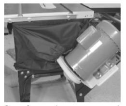
8) Before starting your saw, crank your blade over to 45 degrees to make sure there is enough material to accommodate this action. You may need to adjust where you have placed the excess material.
