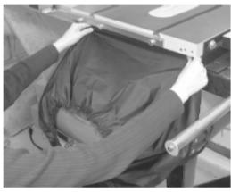
4) With the top side up (side with the stiffener), slip 'The Boot' over the motor and belt guard.
