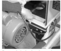
3) Attach the hook & loop strips to the sides and bottom of the saw body by peeling the protective back off the velcro strip. Rub firmly so it fastens well to the saw body.
