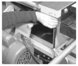
2) Measure the length of each side of the saw body and the bottom of the opening. Cut hook & loop strips to these measurements.
