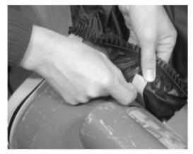
7) Fasten the small hook & loop strip (found inside 'The Boot') to the motor or belt guard (whatever works best on your saw). This will stop 'The Boot' from being sucked into the back of the saw when the dust collector is on.
