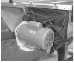
5) There is a hook & loop strip attached inside 'The Boot'. Attach 'The Boot' hook & loop strip to the strips you just applied to your saw body.
