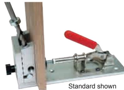
**Start the drill bit into the guide bushing and just before you make contact with the wood, pull the trigger of the drill to bring the RPM of the drill bit up to full speed before touching the material.**
